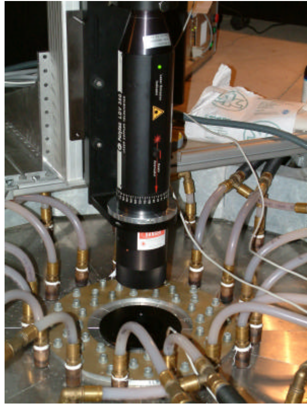
Fig.2: Schematic sketch (left) of the cylindrical convection cell with heating plate on the bottom (red) and cooling plate at the top (blue). LDA and temperature measurements (right) are accomplished through a glass window in the center of the cooling plate.
