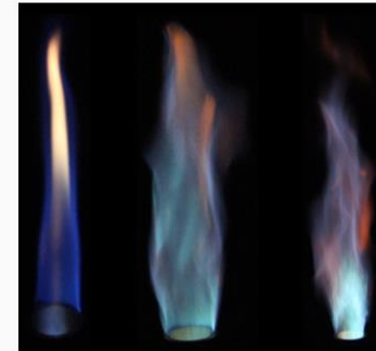
PICTURE 2 – STABILITY LIMITS OF A TURBULENT FLAME
